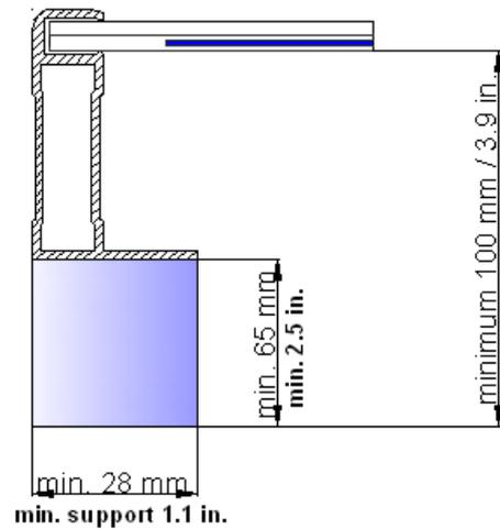
In case of installation on a pitch, it is advisable to keep a distance of at least 10 cm from the underlying area to allow adequate ventilation of the rear of the module.
